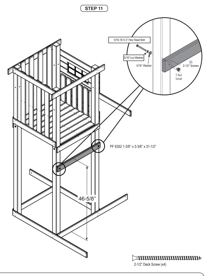
1. Attach Frame Support Board as shown.
