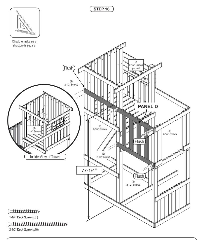
1. Attach Panel D to Frame A as shown.
