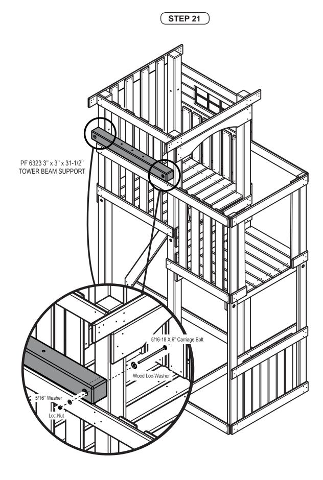
1. Attach Tower Beam Support Board as shown.
