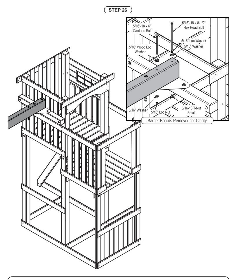
1. Install Swing Beam as shown.
