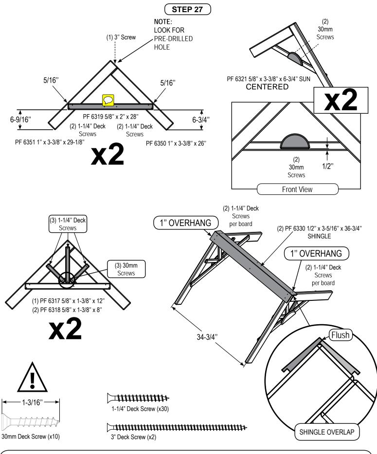
1. Assemble Roof Frame as shown. **NOTE:** Overlap Shingles as shown.
