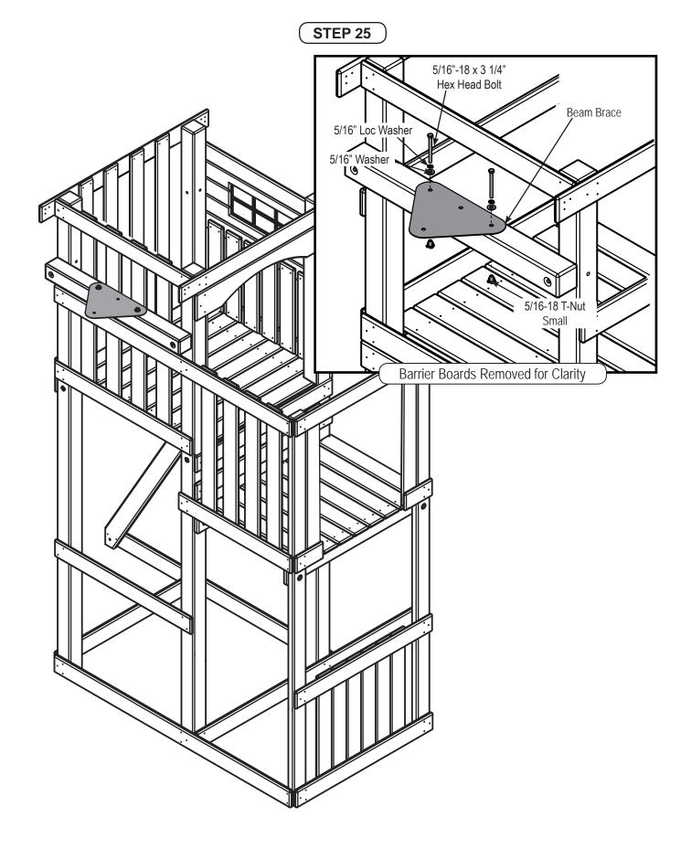
1. Install Swing Beam Brace as shown.
