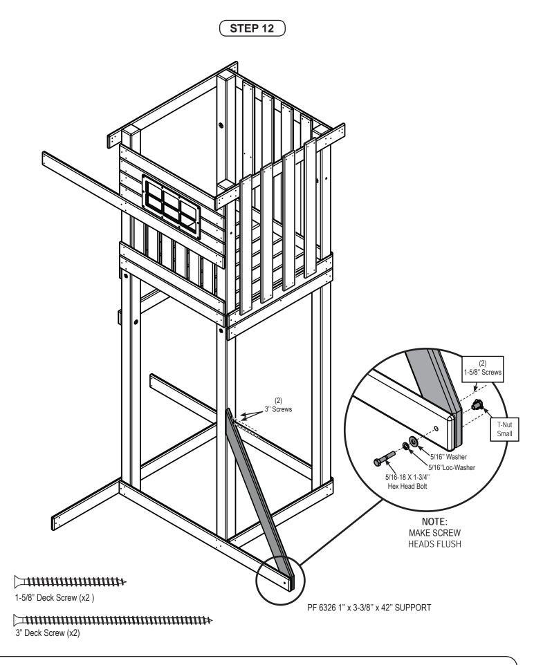
1. Attach Tower Support Board as shown.
