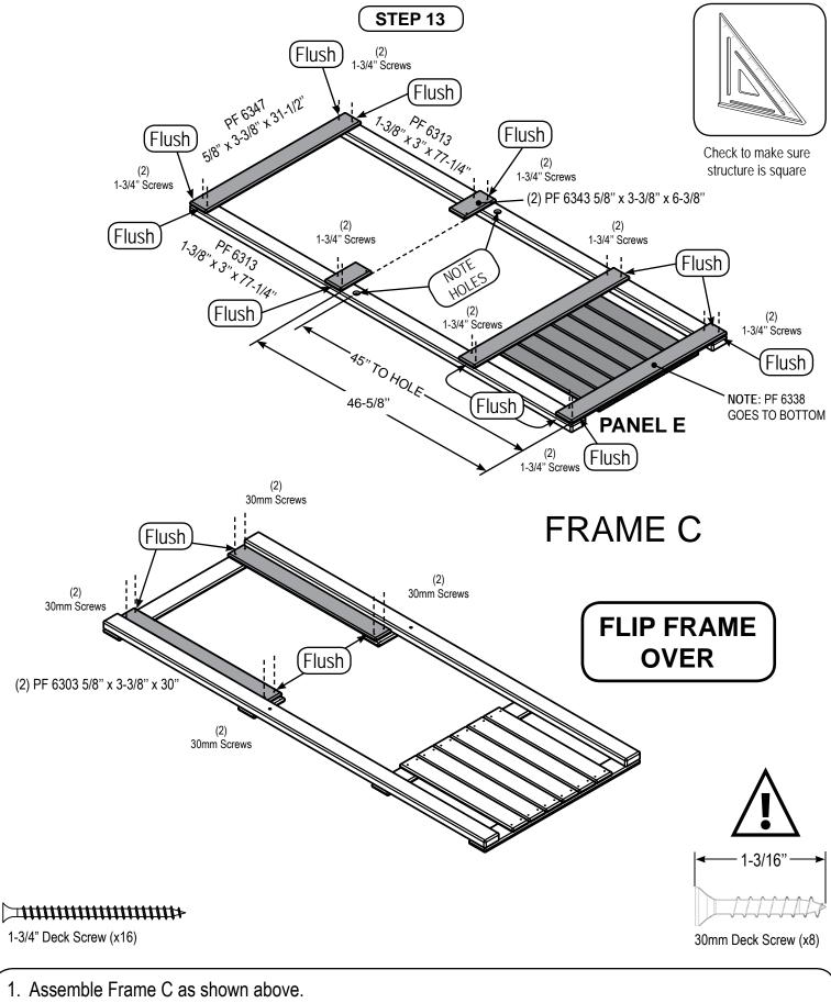
2. Attach barrier boards as shown.
