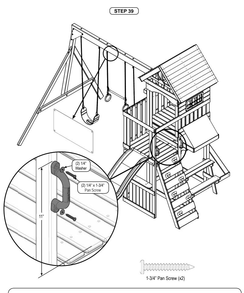
1. Attach Safety Handle and Name Plate as shown.
