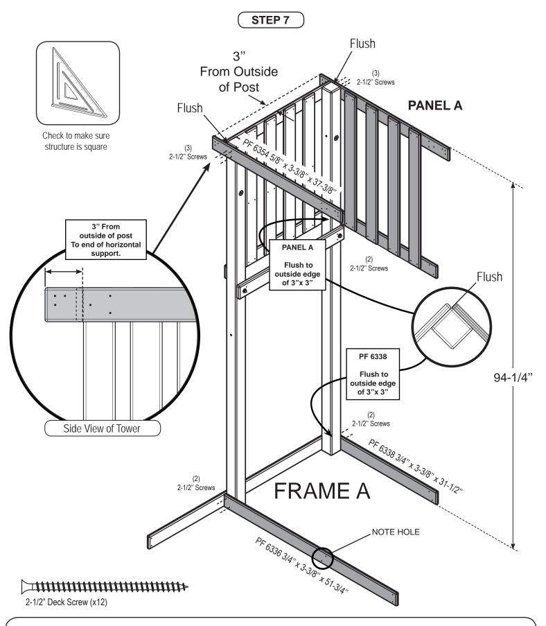
1. Attach frame Support Boards and Panel A to Frame A as shown above.
