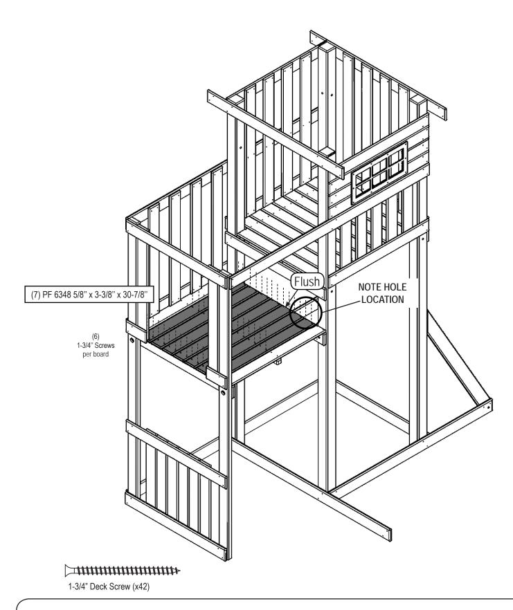
Install Deck Boards as shown. NOTE: Standard gap between deck boards is 1/8".
