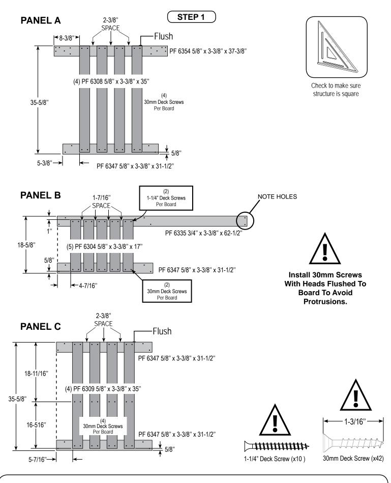
1. Assemble Panel A, Panel B and Panel C as shown.
