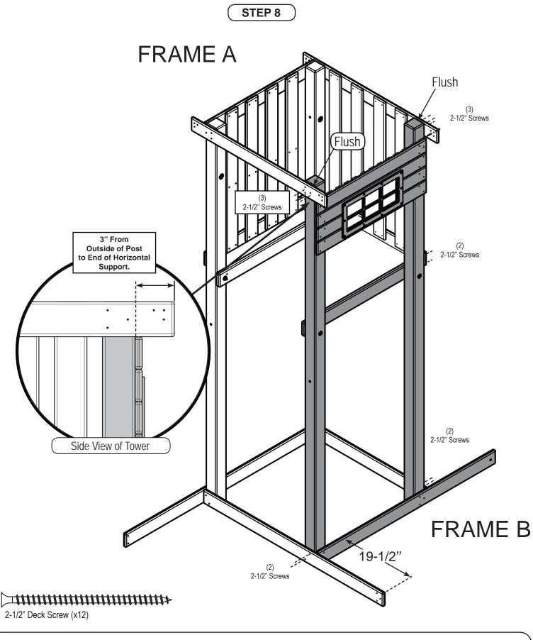
1. Attach Frame B to Frame A as shown.
